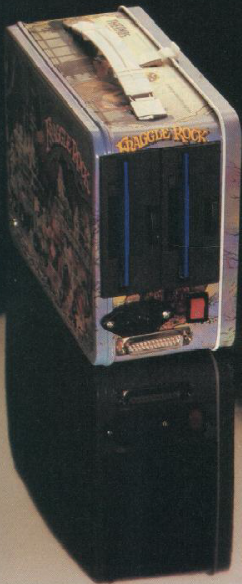
Photo 1: A standard lunchbox can be converted into a powerful computer with the SB180.
