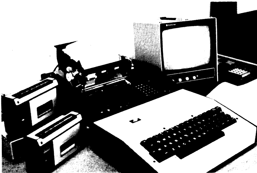
KIM-1 and KIM-2 in redwood enclosure, ACT-1 TVT, Telpar Printer, Computerist power supply, Radio Shack recorders.
