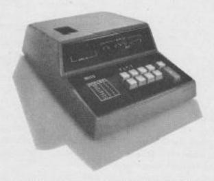
The Altair VLCT is ideal for machine language programming. It converts a three digit octal code directly into an 8 digit binary code for transmission to the computer and then displays the binary output from the computer in a 3 digital octal format. This allows you to program in octal which is much easier than programming in binary. In addition, the VLCT is much more convenient to work with than using the front panel switches of the Altair 8800.
